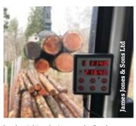
Load weighing devices may be fitted to lorry-mounted loaders.
