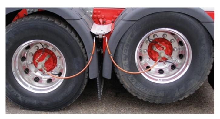
Tyre pressure control systems fitted to timber lorries can help reduce the impact on fragile roads.
