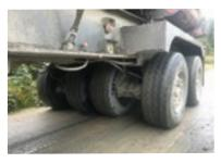
This bespoke low ground pressure timber vehicle spreads the weight of the load across the road.
